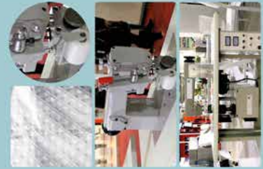
Design and Manufacture of Ultrasonic Sewing Machines with Width up to 20 mm
